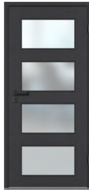
2 NORMTÜR NT-LA11-DA G-TEC® Graphitgrau Matt 7024 GLAS SATINATO, Standard-Ornamentglas ZARGE KR1 BESCHLAG CUBO, Graphitschwarz MODEL STANDARD DOOR NT-LA11-DA FINISH G-TEC® Matte Graphite Grey 7024 GLASS SATINATO, standard patterned glass FRAME KR1 FITTINGS CUBO, Graphite black
